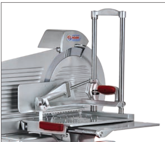
NS300V and NS330M - feature double sliding plate with lockable hand grip to securely hold meat in place.
